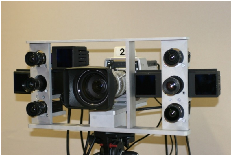
Camera rig with 5 color cameras + 2 ToF depth cameras (left/right)
