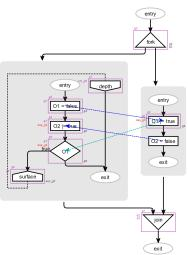
Basic blocks may be interrupted when a data dependency interferes.
