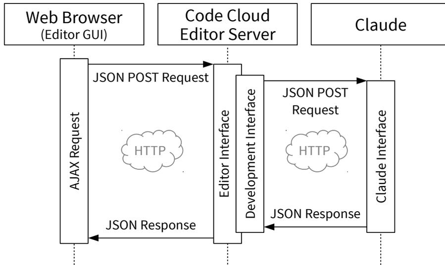
Figure 3.17. AJAX communication of the different editor components
