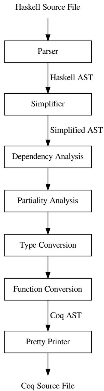
**Figure 4.1.** Stages of the compilation process from Haskell to Coq. Arrows are labeled with the intermediate representation of the data passed between two stages.
