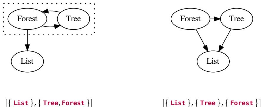
**Figure 3.6.** Dependency graphs for **Tree** and **Forest** before inlining the type synonym **Forest** into the definition of **Tree** (left) and after inlining (right). Strongly connected components are listed in reverse topological order below the graphs.
