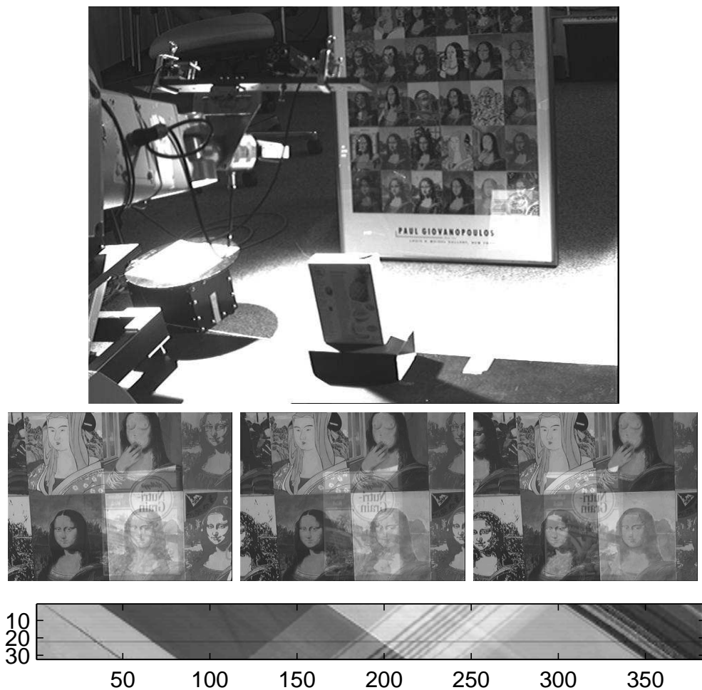
Figure 4.9: Real transparency sequence. Row 1: This image displays how we produce the transparency sequence. We move the camera and the muesli package separately to produce two independent motions. The left moving muesli package is reflected on the glass of the portrait so that we obtain a transparency sequence. Row 2: The first, 16-th and 32-th frames of the image sequence. Each frame has 288 \times 384 pixels. We use the 16-th frame for motion estimation and scene analysis. Row 3: Epipolar slide of the whole image sequence volume at the 150-th row. We can see the transparent motions clearly as the overlapping of two tilted structures.
