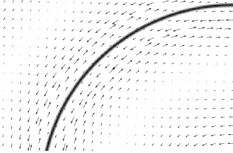
Figure 4: Monogenic phase of a simple image. The phase is represented by the vector field and the image (arc) is represented by the grayscale pattern. Note also the phase-wrapping.
