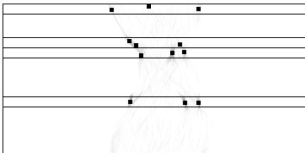
FIG. 31: Result of applying the windowed OHT to the quadrangle image window in Fig. 20 and selecting 12 Hough peaks organized in four stripes of respective three Hough peaks.
