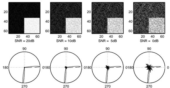
Figure 4: **Top:** A synthetic edge junction disturbed by incremental random noise. **Bottom:** Corresponding *Differentiation outputs*  $h(\theta)$ . Even in the very noisy case ( $SNR = 0dB$ ) we can still match the junction.  $W = 10^\circ$ ,  $R = 9$ ,  $S = 11$ .
