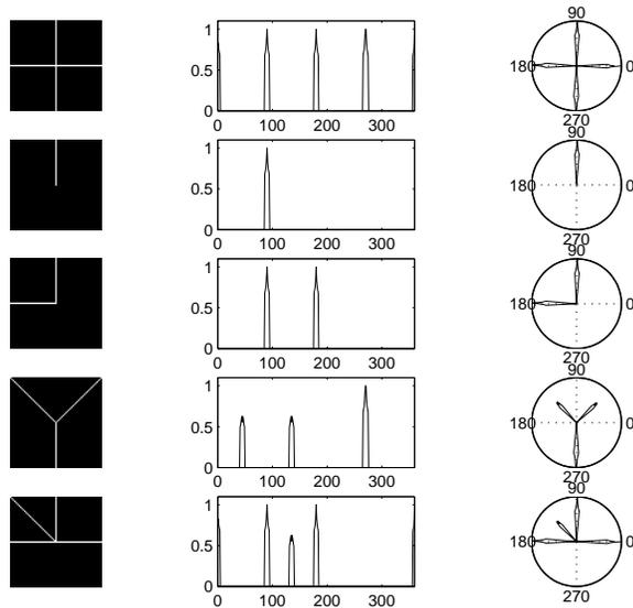
Figure 2: **Left:** Synthetic line junction images with the size of  $65 \times 65$  pixels and line width of 1 pixel. **Middle:** *Averaging outputs*  $g(\theta)$  v.s.  $\theta$  from  $0^\circ$  to  $360^\circ$ .  $W = 8^\circ$ ,  $R = 15$ . The positions of the local maxima exhibit the orientations of lines. **Right:** Corresponding polar plots of the results in the middle column. The numbers around circles are angles in degree.
