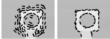
Fig. 1. The very right image shows the original face image I , the other images show the image I , represented with 16, 52, 116 and 216 Gabor wavelets (left to right). In the very left image, the positions of the first 16 wavelets are indicated.
