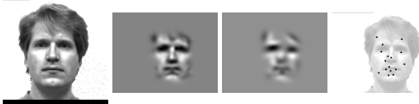
Figure 1. A GWN with N = 52 wavelets is optimized for image I (very left) according to eq. (2). The second image (from left) shows the corresponding GWT \hat{I} . The third image shows the GWT \hat{I}_{16} , made up of just the 16 largest wavelets, the fourth image shows their positions.
