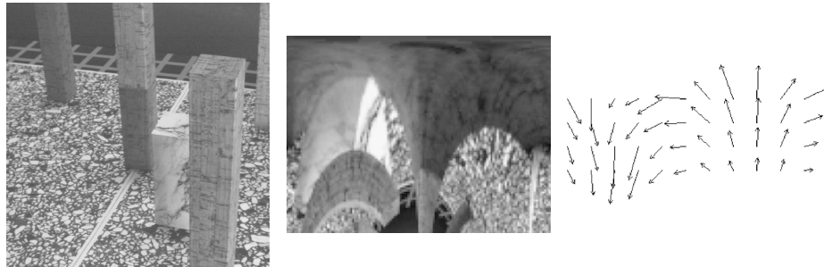
Fig. 2. The cartesian original image 512x512 pixels(left), its log-polar transform 77x128 pixels shown magnified (middle), and the computed optical flow (right) of the “Marbled Block” sequence. The horizontal axis is the angular axis and the vertical axis is the logarithmic radial axis.
