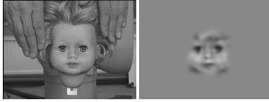
Figure 6: The left image shows the original doll face image I , the right image shows its reconstruction \hat{I}_{4,6} using the reconstruction formula with an optimal wavelet net \Psi of just N = 52 odd Gabor wavelets, distributed over the inner face region. For optimization, the scheme that was introduced in section 2 was applied.
