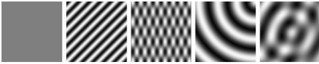
Fig. 3 From left to right: a constant signal (i0D), an arbitrary rotated 1D signal (i1D) and an i2D checkerboard signal consisting of two simple superimposed i1D signals. A curved i2D signal and two superimposed curved i2D signals. Note that all signals displayed here preserve their intrinsic dimension globally
