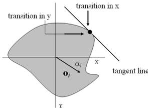
**Figure 2. The transition index is determined according to the position of the normalized orientation vector in image coordinates and the object assumption (dark object on a bright background).**
