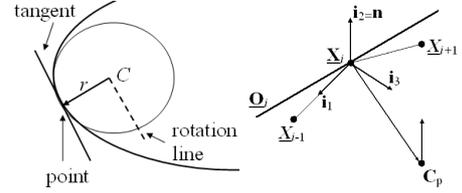
**Figure 1. Left figure: local rotor for a 3D contour, right figure: local coordinate system needed to get the circle parameters and the motor.**
