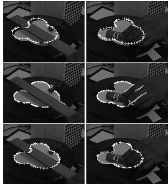
**Figure 4. The top images show the initial pose, the middle row shows the detected segments and the bottom row shows the pose results.**
