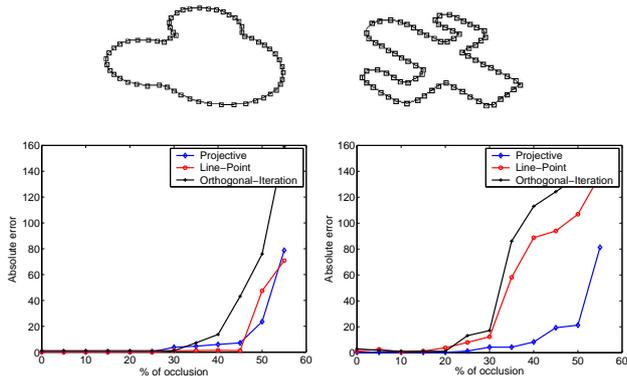
**Figure 3. Absolute error in millimeters for the mouse model (left) and the cactus model (right) while increasing the occlusion.**
