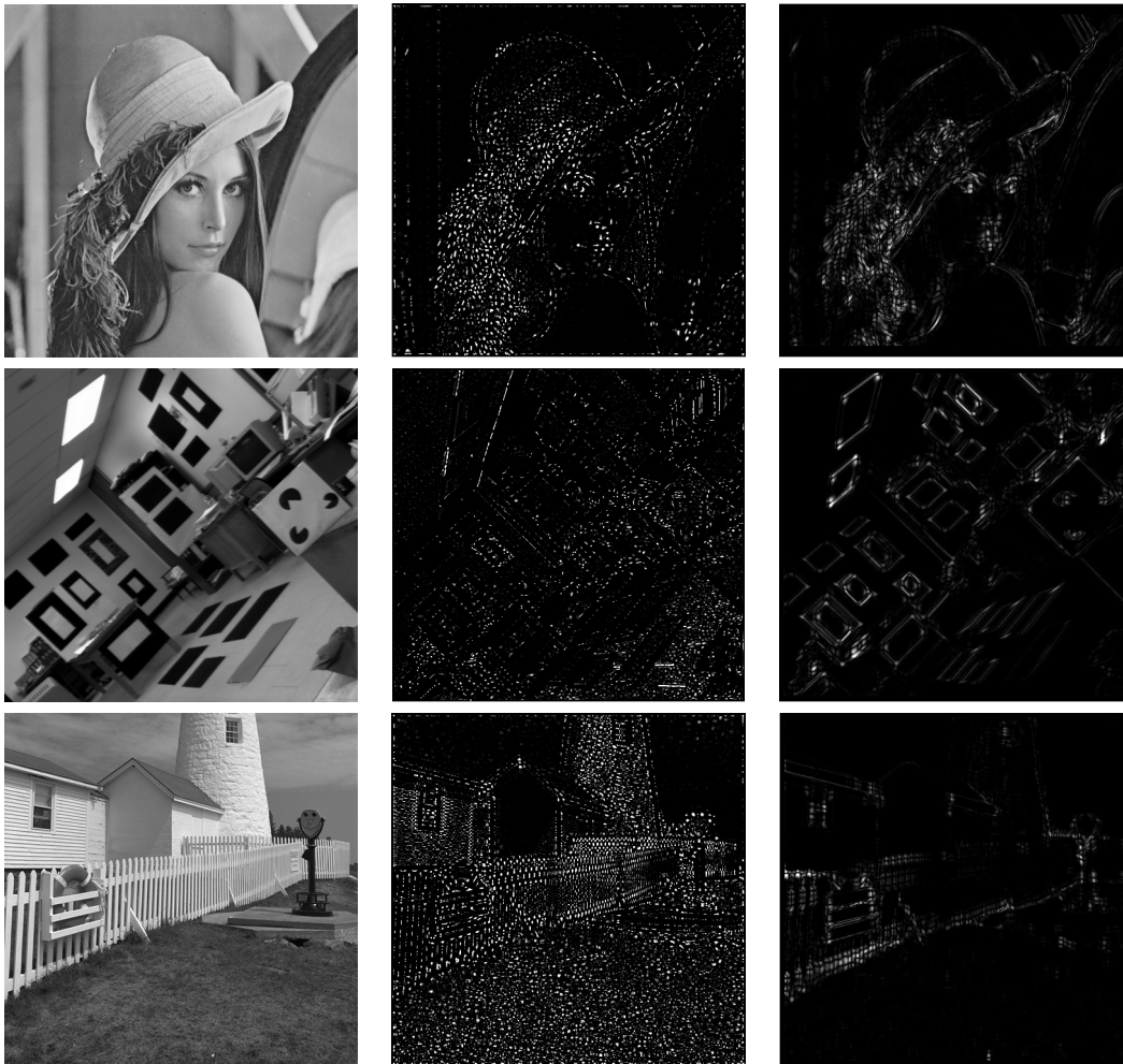
Figure 5.19: Left: Original test images Middle: Gaussian curvature calculated with finite differences in Poisson scale space ( s=2.0 ) Right: Gaussian curvature calculated with the conformal monogenic signal method and filter mask size 15 pixel( s=2.0 )
