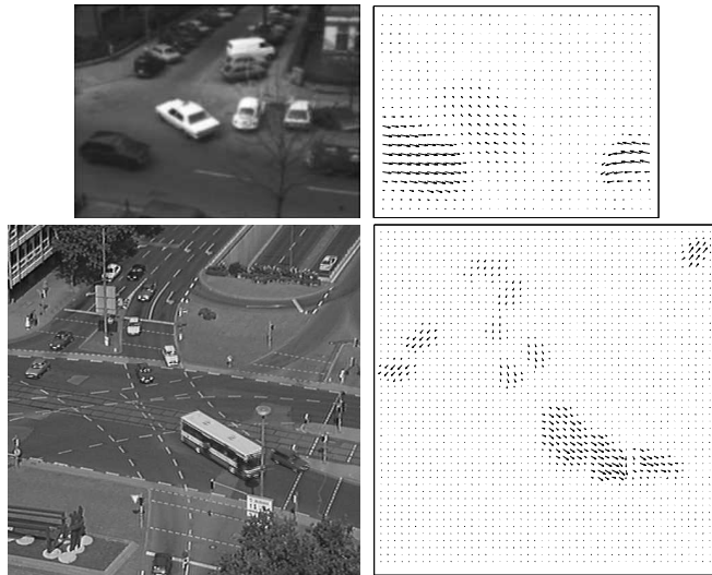
Fig. 6. Top row: one frame of the Hamburg taxi sequence and the estimated optical flow from our approach. Bottom row: one frame of the Ettliger Tor traffic sequence and the flow fields from our approach.
