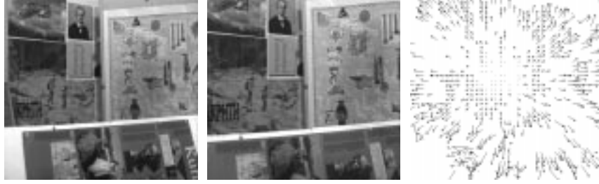
Fig. 6. The 1st (left) and the 10th (middle) of the real fixated sequence and the computed optical flow field (right)
