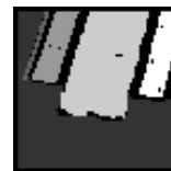
Figure 6: Gripper patch with grasped object and its segmentation image.
