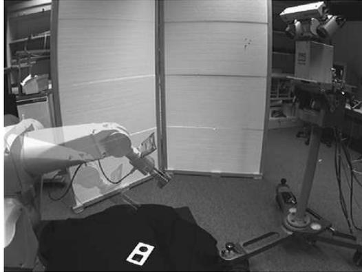
Fig. 1. Robot head and manipulator, approaching an object towards a camera for shape inspection.
