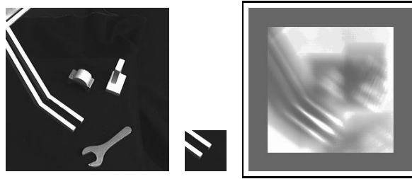
Figure 13: Scene, gripper image region and resulting correlation image.
