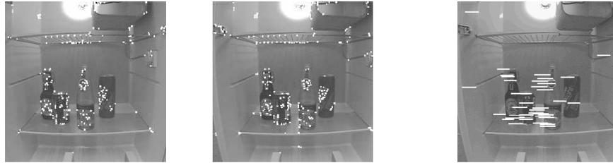
**Fig. 1.** (a) and (b) Two consecutive images with gray value corners: (c) Image with motion vectors at the gray value corners.
