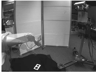
Fig. 1. Robot head, manipulator; approach an object towards a camera for shape inspection.
