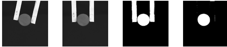
Fig. 5. (a) Appropriate size of depicted situation; (b) Vertical appearance of robot fingers; (c) Binary image with object and fingers; (d) Extraction of grasped object.
