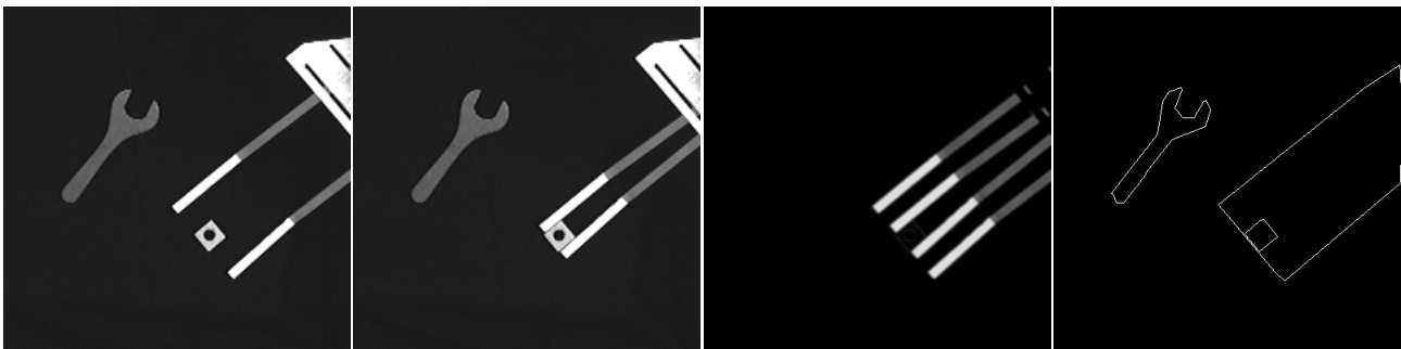
Figure 3: Image of the scene with opened gripper, image of the scene with closed gripper, difference image, contour of the grasped object and the target object with the convex hull which describes the gripper range.
