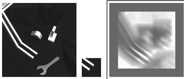
Figure 3: Scene, gripper image region and resulting correlation image (higher greylevel indicates better correlation)
