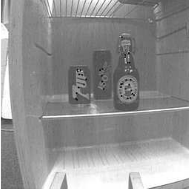
Figure 2: Detected grey level corners at two obstacle objects (left and right) and one goal object (middle).
