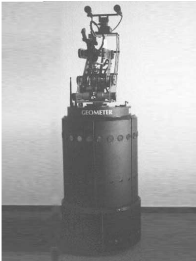
Fig. 1. The experimental robot equipped with sonar, IR, tactile sensors, and an odometry system. The six DOF manipulator and the binocular CCD camera are reserved for visual processing.
