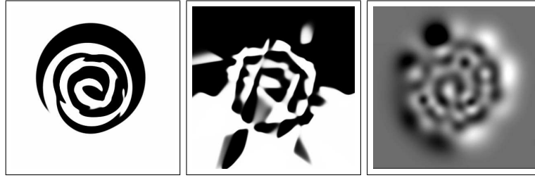
Fig. 1. Two spirals benchmark. Visualization of nearly perfect classification for different network types. White and black colors represent the two classes, that are to be learned. Gray color represents an area of unreliable decision. Left - MLHP with 10 neurons in hidden layer; Middle - MLP with 60 neurons in hidden layer; Right - RBF with 80 neurons in hidden layer.
