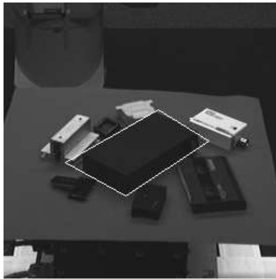
Fig. 2.24. The silhouette boundary of the dummy box is included in the set of most conspicuous, approximate parallelograms.
