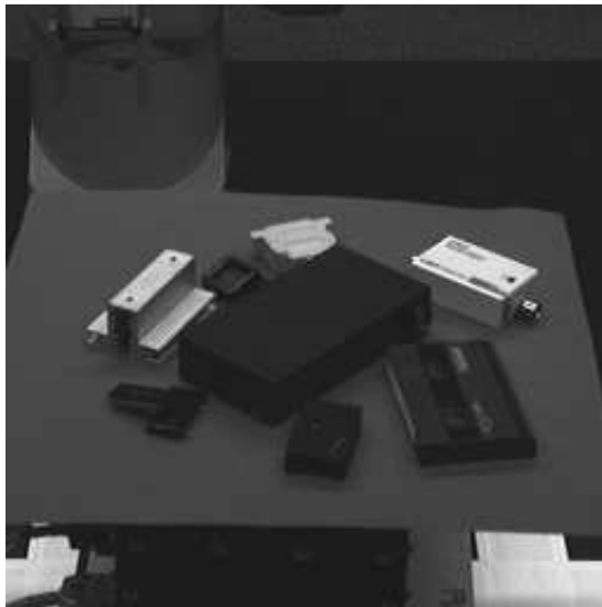
Fig. 2.15. Arrangement of objects in a scene of electrical scrap. The black dummy box is our target object for the purpose of demonstration. It is located in a complex environment, is partially occluded, and has a protruding socket.
