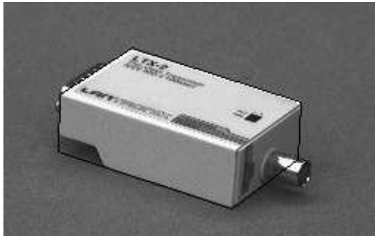
Fig. 2.43. Extracted regular hexagon, which describes the approximate silhouette of the transceiver box.
