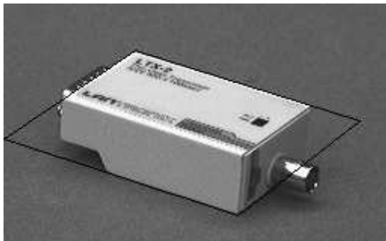
Fig. 2.42. Transceiver box with approximate right-angled parallelepiped shape. The black quadrangle surrounding the object indicates the image window for detailed processing.
