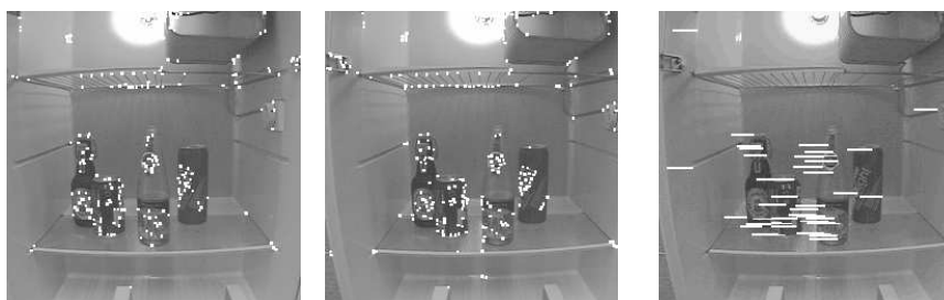
Fig. 4.14. Extracting gray value corners in two consecutive images; detecting correspondences.
