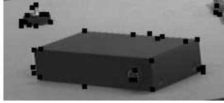
Fig. 2.10. The SUSAN operator has detected a set of gray value corners shown as black squares. We find all those gray value corners included which are characteristic for the three-dimensional object boundary.
