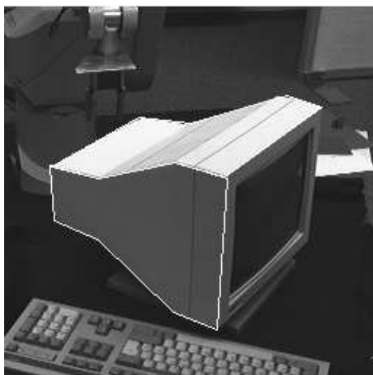
Fig. 2.29. Computer monitor with two types of regularities of the polygonal faces. The side face is approximate reflection-symmetric, and the top face is approximate translation-symmetric.
