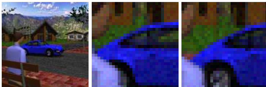
Figure 1.1: Problems in Matching: Occlusion and Depth Discontinuities (Rear Wheel), Noise and Invariance (Door Handle), Aperture Problem (Lower Window Edge)
