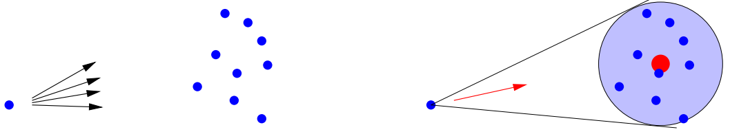
Figure 1.1: Replacing a cluster of stars by a “virtual star” that exerts approximately the same gravitational force
