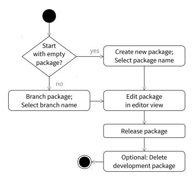
Figure 3.10. Workflow to develop a new package
