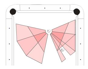
Figure 2.8: Polygons created for shape zone approximation
