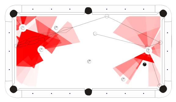
Figure 2.10: Crossing zones created for shape zone approximation on a sample shot
